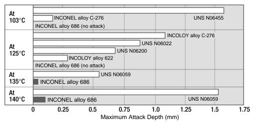
Figure 30 – Relative resistance of nickel-based alloys to crevice corrosion as a function of temperature in 11.9%  $H_2SO_4 + 1.3\%$  HCl + 1% FeCl<sub>3</sub> + 1% CuCl<sub>2</sub>.
