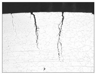
Figure 48 - Transgranular cracking in an austenitic stainless steel U-bend specimen exposed for 8 days to boiling 42% MgCl<sub>2</sub> vapors. Etchant, glyceregia. (70X)
