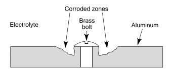
Figure 47 - Galvanic corrosion.
