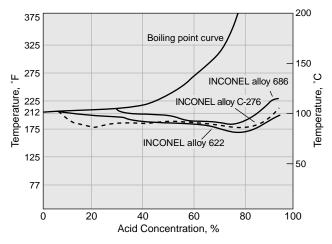
Figure 4 – Comparative behavior of Ni-Cr-Mo alloys in sulfuric acid. The iso-corrosion lines indicate a corrosion rate of 20 mpy (0.51 mm/a).
