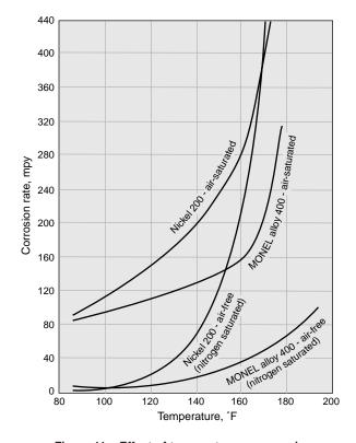
Figure 10 - Corrosion of Nickel 200 and MONEL alloy 400 in hydrochloric acid solutions at 86°F (30°C).
