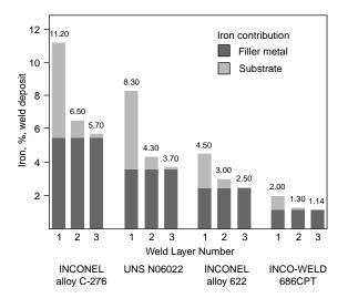
Figure 36 - Effect of filler metal composition on iron content for Ni-Cr-Mo alloys overlayed on steel by the GMAW process.
