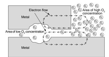
Figure 46 - Corrosion resulting from oxygen concentration.
