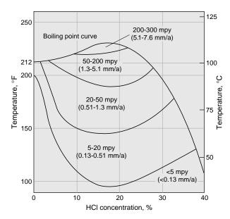
Figure 14 – Iso-corrosion chart for INCONEL alloy C-276 in hydrochloric acid.
