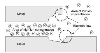
Figure 45 - Corrosion resulting from metal-ion concentration.
