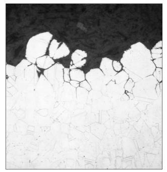
Figure 52 - Intergranular corrosion. (200X)
