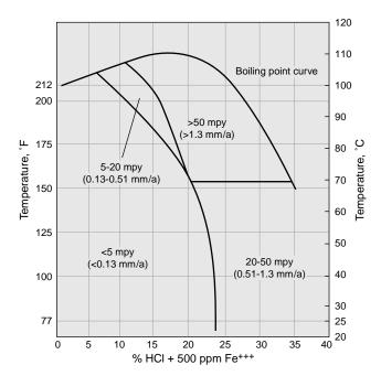
Figure 15 – Iso-corrosion chart for INCONEL alloy 686 in hydrochloric acid + 500 ppm Fe<sup>+++</sup>.
