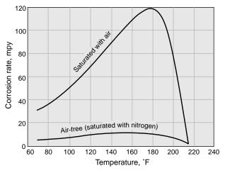
Figure 1 – Effect of temperature on corrosion of MONEL alloy 400 in sulfuric acid. Acid concentration, 5-6%. Velocity, 15.5-16.5 ft/min.
