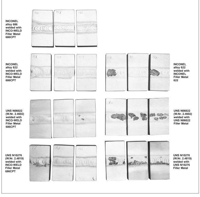
Figure 35 - Pitting-resistance of base metal/weld metal combinations. Exposed for 3 days at 217°F (103°C) in 11.9%  $H_2SO_4$  + 1.3% HCl + 1% FeCl<sub>3</sub> + 1% CuCl<sub>2</sub>.
