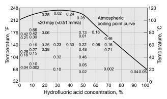
Figure 22 – Corrosion data for MONEL alloy 400 in hydrofluoric acid. Corrosion rates are shown in mm/a.
