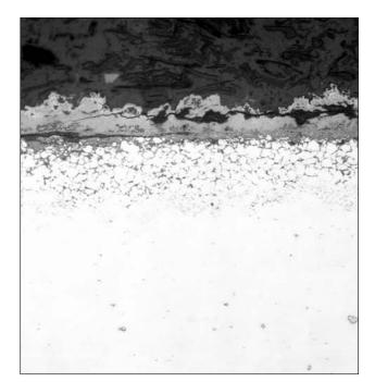
Figure 53 - Intergranular oxidation. (200X)
