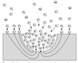
Figure 44 - Autocatalytic process occuring in a corrosion pit.
