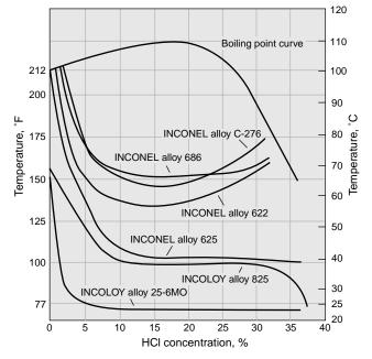
Figure 19 – Comparative behavior of nickel-based alloys in hydrochloric acid. The iso-corrosion lines indicate a corrosion rate of 20 mpy (0.51 mm/a).
