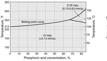
Figure 26 - Iso-corrosion chart for INCONEL alloy C-276 in phosphoric acid.
