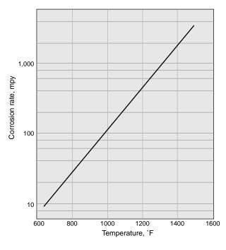
Figure 34 - Corrosion of INCONEL alloy 600 in dry hydrogen chloride gas. Rates converted from inches per month.
