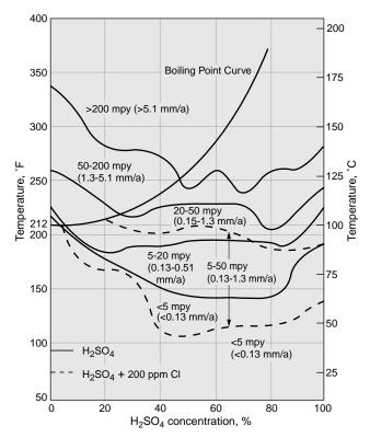
Figure 6 – Iso-corrosion chart for INCONEL alloy C-276 in sulfuric acid.
