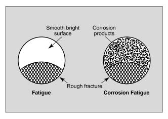
Figure 51 - Schematic illustration of fatigue and corrosion-fatigue failures.
