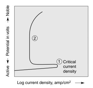
Figure 41 - Polarization curve for a passive metal anode. (1) maximum current and maximum corrosion. (2) passive state. Current at (2) can be hundreds or thousands of times smaller than (1).
