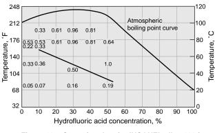
Figure 23 – Corrosion data for INCONEL alloy 600 in hydrofluoric acid. Corrosion rates are shown in mm/a.
