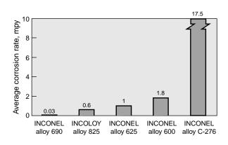
Figure 28 – Average corrosion rates for nickel alloys in 10% nitric acid at boiling temperatures.
