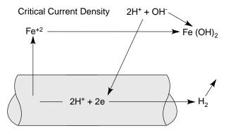
Figure 40 - Corrosion of iron in water.
