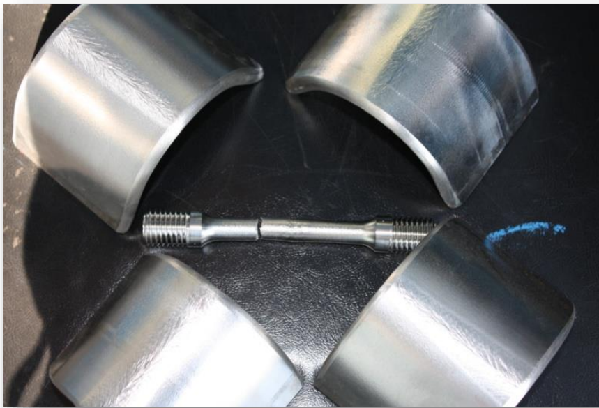
Figure 18. Full-section, direct-aged 4T side bend test specimens from the HWGTAW steam header tube weldment. The room temperature tensile specimen fractured in the base metal away from the weld.
