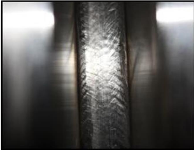
Figure 15. HWGTA weld in progress in large diameter, heavy wall INCONEL alloy 740H tube to simulate fabrication of an A-USC boiler steam header.
