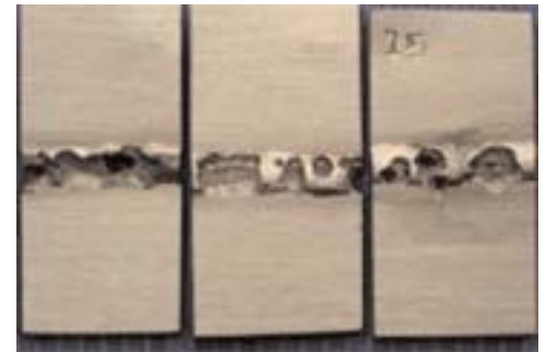
Hastelloy C-2000 alloy welded with matching filler metal.
