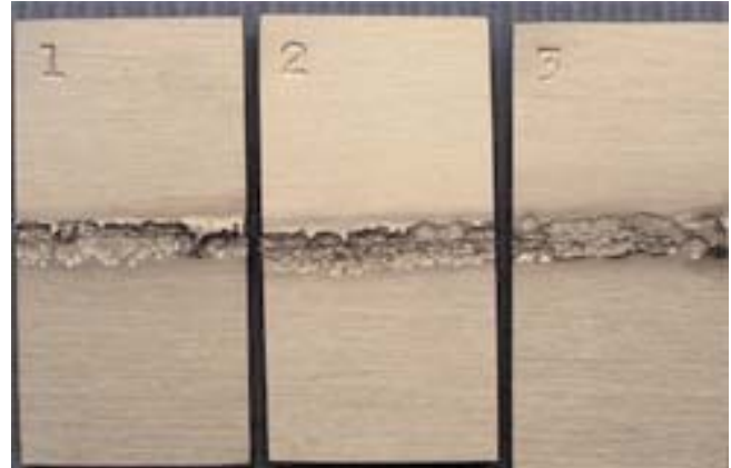
INCONEL alloy C-276 welded with matching filler metal.
