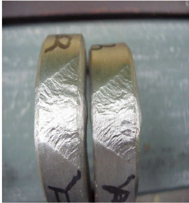
Figure 9. Side bends performed on as-welded butt joint, joining 8mm INCONEL alloy 693 plate using INCONEL filler metal 52 and capping at the root and face with INCONEL filler metal 72.
