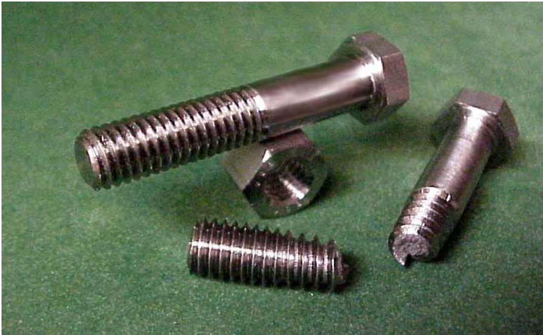
FIGURE 3 5/16 in. (14 mm) x 16 Nut and Bolts Tested per ASTM Standard Practice F606.
