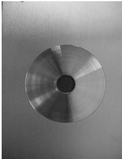
Figure 8: Unattacked sample of 27-7MO after 60-day exposure to seawater with crevice.
