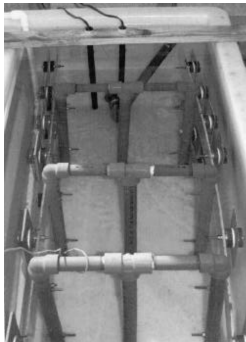
Figure 5: The setup used for crevice corrosion testing in seawater.
