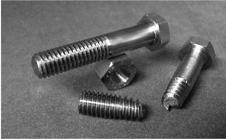
FIGURE 3 – INCONEL alloy 686 5/16 in. X 16 Bolts and Nut. The fracture surface of the bolt broken during tensile testing exhibits ductile fracture .
