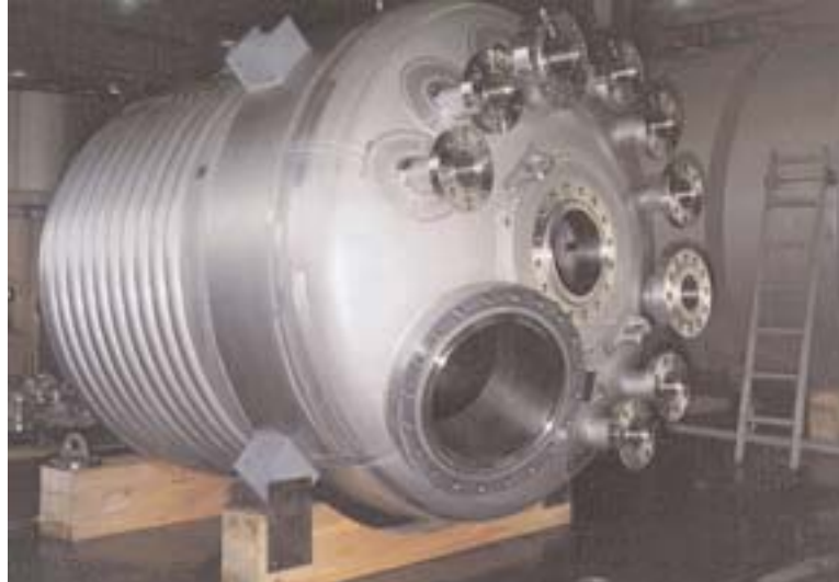
Multi-purpose pharmaceutical vessel manufactured in 40mm thick INCONEL alloy 686 plate.
