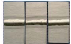
INCONEL alloy 22 with INCO-WELD FM 686CPT
