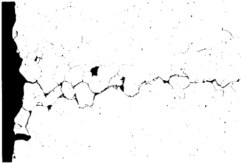
Figure 1. Intergranular PTA SCC produced in Type 347 Stainless Steel reformer tube. Heavy intergranular carbide precipitation was present, apparently as the result of improper heat treatment. Magnification 100X, Etchant: 10% oxalic, electrolytic
