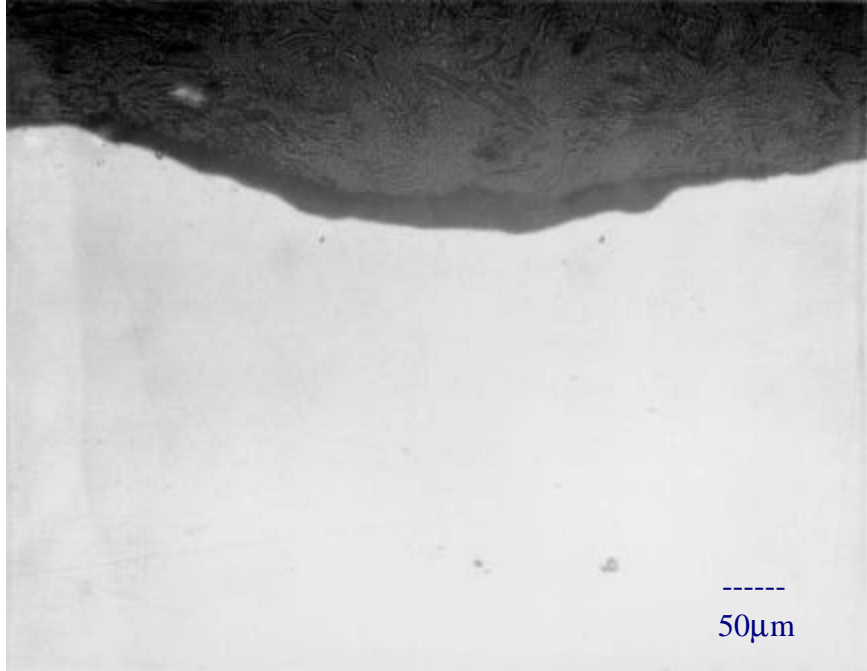
Figure 11. Photomicrograph showing cross section of alloy 686 sample after exposure for 336 hours in N_2 -10% O_2 -10% CO_2 -20% H_2O -1500ppm HCl-300ppm SO_2 at 550°C. Sample was painted with ash 1. Unetched.
