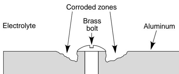
Figure 47 - Galvanic corrosion.
