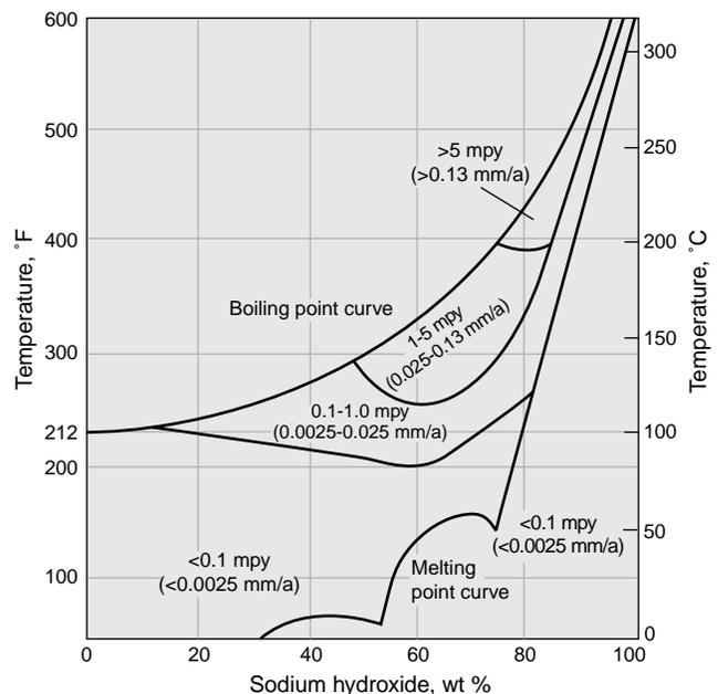
Figure 29 – Iso-corrosion chart for Nickel 200 and 201 in sodium hydroxide.
