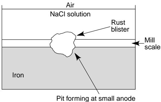
Figure 43 - Pitting at break in mill scale.
