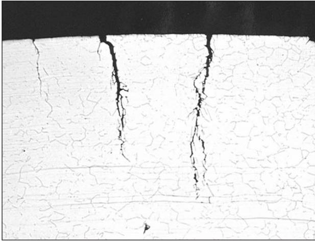
**Figure 48 - Transgranular cracking in an austenitic stainless steel U-bend specimen exposed for 8 days to boiling 42% MgCl<sub>2</sub> vapors. Etchant, glyceresia. (70X)**
