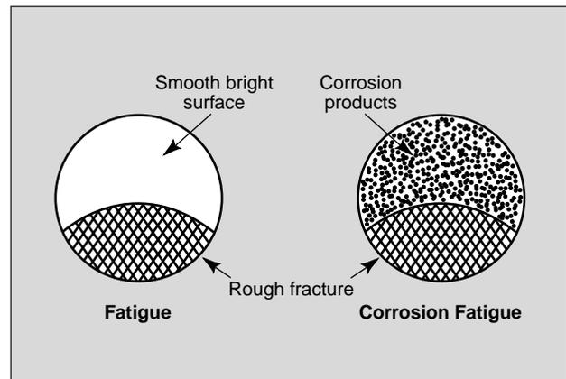
**Figure 51 - Schematic illustration of fatigue and corrosion-fatigue failures.**
