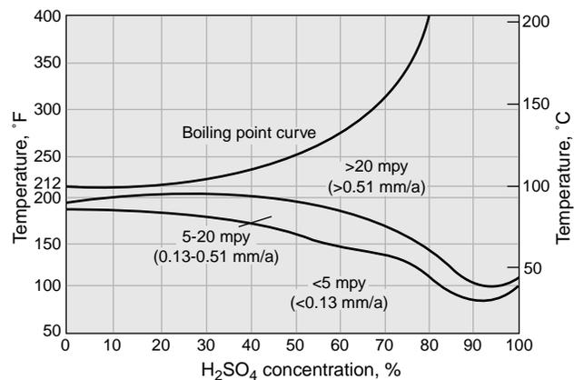
Figure 8 – Iso-corrosion chart for INCONEL alloy 625 in sulfuric acid.
