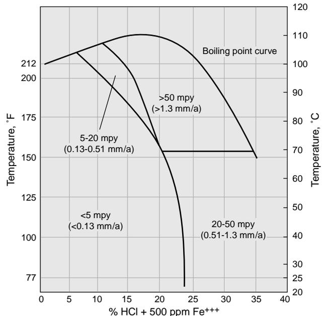
Figure 15 – Iso-corrosion chart for INCONEL alloy 686 in hydrochloric acid + 500 ppm Fe<sup>+++</sup>.
