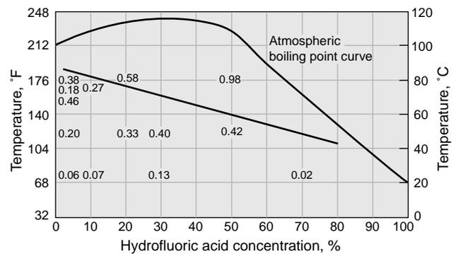
Figure 20 – Corrosion data for Nickel 200 in hydrofluoric acid. Corrosion rates are shown in mm/a.
