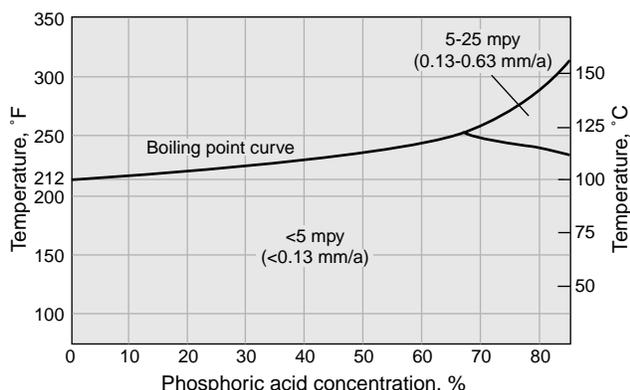
Figure 26 – Iso-corrosion chart for INCONEL alloy C-276 in phosphoric acid.
