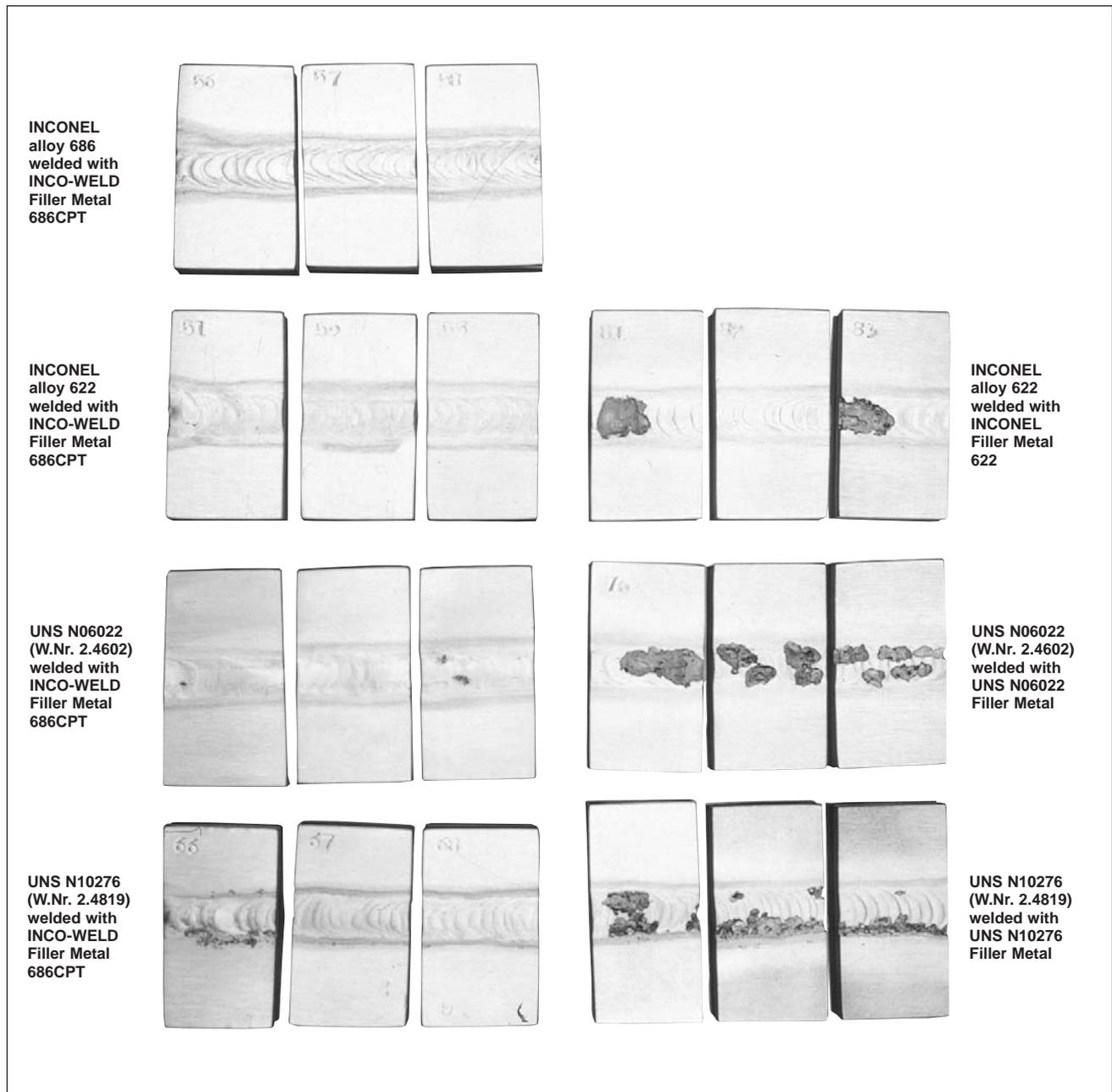
**Figure 35 - Pitting-resistance of base metal/weld metal combinations.**
