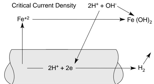
Figure 40 - Corrosion of iron in water.
