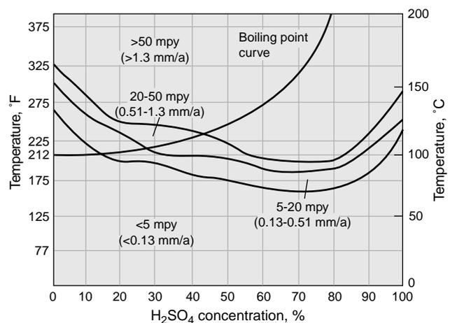
Figure 9 – Iso-corrosion chart for INCONEL alloy 686 in sulfuric acid.
