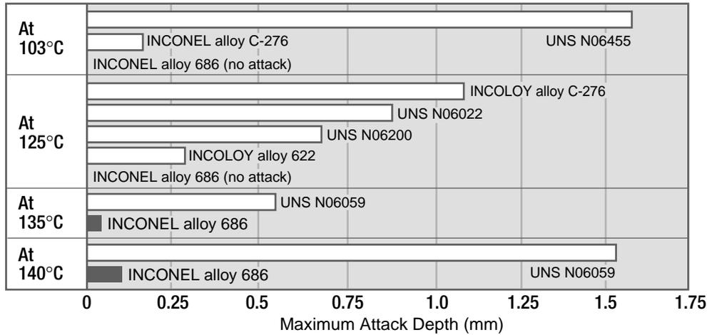
Figure 30 – Relative resistance of nickel-based alloys to crevice corrosion as a function of temperature in 11.9% H<sub>2</sub>SO<sub>4</sub> + 1.3% HCl + 1% FeCl<sub>3</sub> + 1% CuCl<sub>2</sub>.
