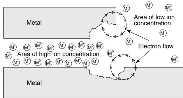
Figure 45 - Corrosion resulting from metal-ion concentration.
