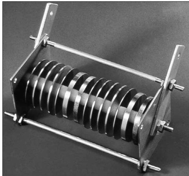
Figure 38 - A typical test coupon assembly for field corrosion testing.
