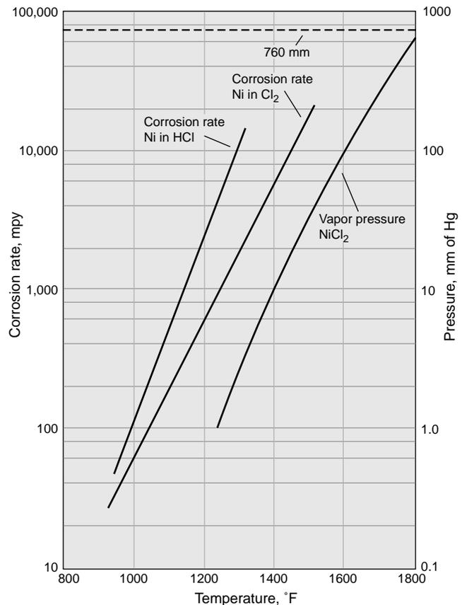
**Figure 32 - Corrosion of nickel in dry chlorine and dry hydrogen chloride. Rates converted from inches per month.**
