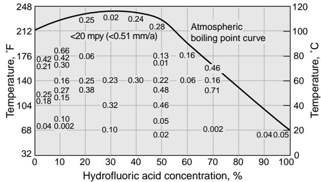
Figure 22 – Corrosion data for MONEL alloy 400 in hydrofluoric acid. Corrosion rates are shown in mm/a.
