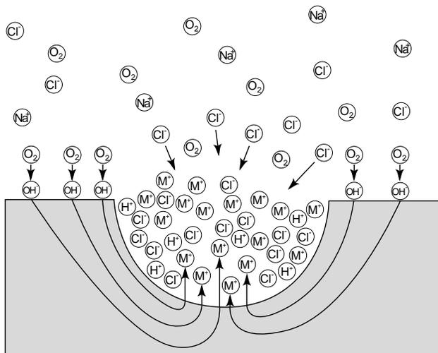
Figure 44 - Autocatalytic process occurring in a corrosion pit.
