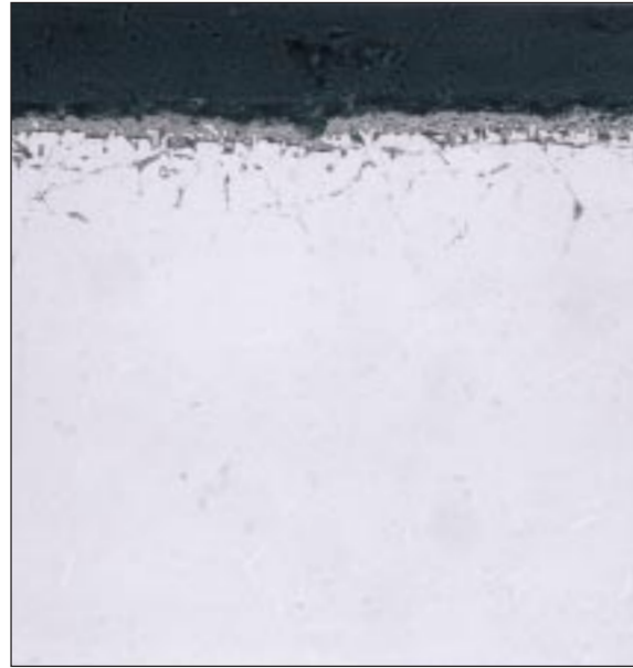
Figure 7 – Photomicrograph of the as-polished cross section of an INCOLOY alloy 864 burner rig sample after 500 h exposure. Magnification: 500X.
