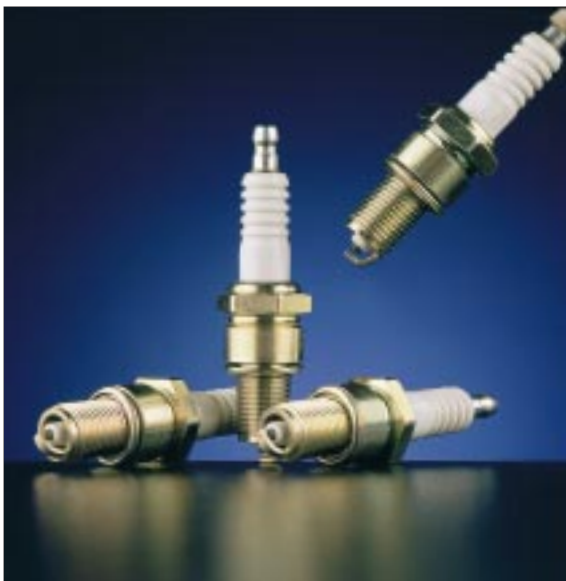
A typical spark plug design where the round center electrode would have a nickel alloy inner core or a nickel-chromium outer layer and a copper alloy inner core, and the rectangular/rhomboidal section ground electrode is in nickel-chromium alloy. Operating temperatures are typically 400 to 900°C (752 to 1652°F).
