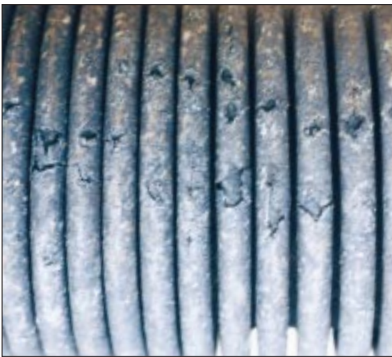
Figure 1 – This two-ply AISI 321 stainless steel bellows failed primarily due to pitting corrosion, general corrosion, and chloride stress-corrosion cracking. INCOLOY alloy 864 and INCONEL alloy 625LCF resist the type of attack illustrated.
