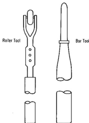
Figure 6. Tools for manual spinning.
