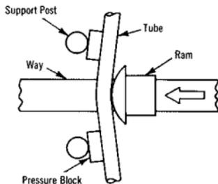
Figure 8. Equipment for press bending.
