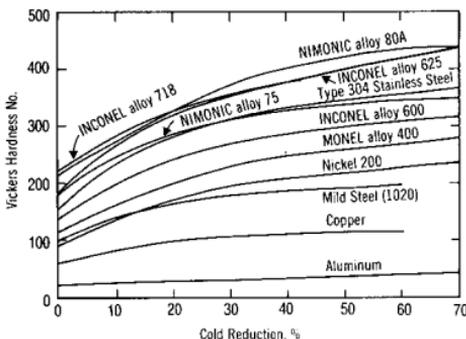
Figure 1. Effect of cold work on hardness.
