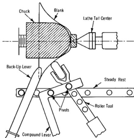
Figure 5. Typical equipment for manual spinning.
