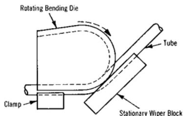
Figure 11. Rotating-die bending with stationary wiper block.
