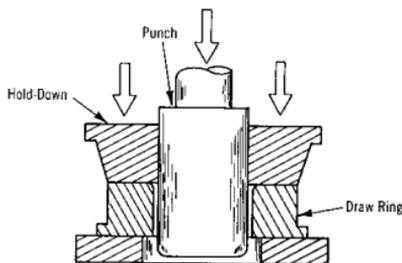
Figure 3. Double-action deep-drawing press.
