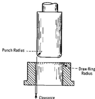
Figure 2. Critical areas in designing deep-drawing equipment.
