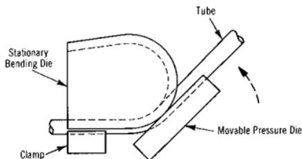
Figure 10. Stationary-die bending.
