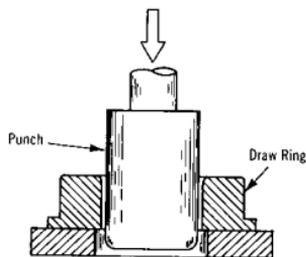
Figure 4. Single-action deep-drawing press without hold-down.
