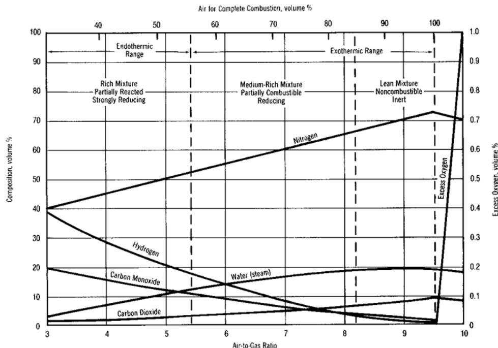
Figure 16. Characteristics and compositions of high-methane natural gas when reacted with air. (Compositions will vary slightly with
