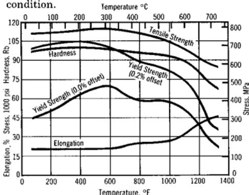
Figure 17. Effect of heating temperature (3 h at temperature) on the room temperature mechanical properties of a MONEL alloy 400 cold-drawn rod.
