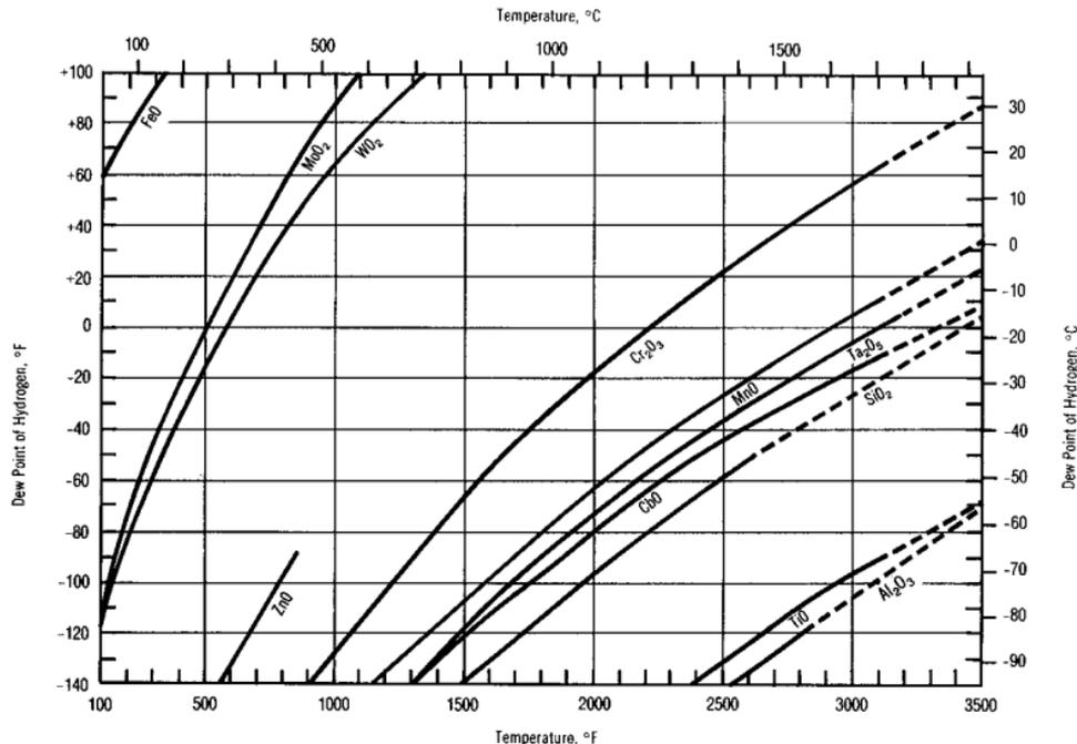
Figure 15. Metal/metal oxide equilibria in hydrogen atmospheres.<sup>1</sup>
