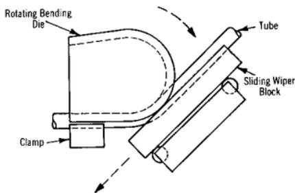
Figure 12. Rotating-die bending with sliding wiper block.
