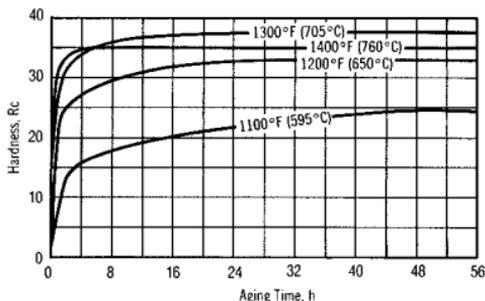
Figure 19. Effect of age hardening at various temperatures on hardness of hot-rolled INCONEL alloy X-750.
