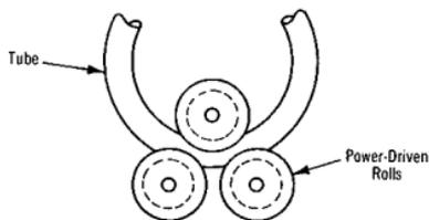
Figure 9. Roll bending. The bend radius is controlled by raising or lowering the top roll.
