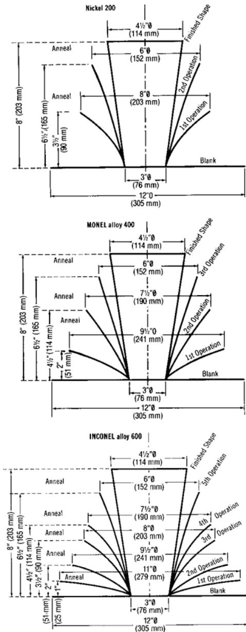
Figure 7. Sequence of operations for spinning deep cups from 0.037 in. (0.94mm) thick blanks of Nickel 200, MONEL alloy 400 and INCONEL alloy 600.
