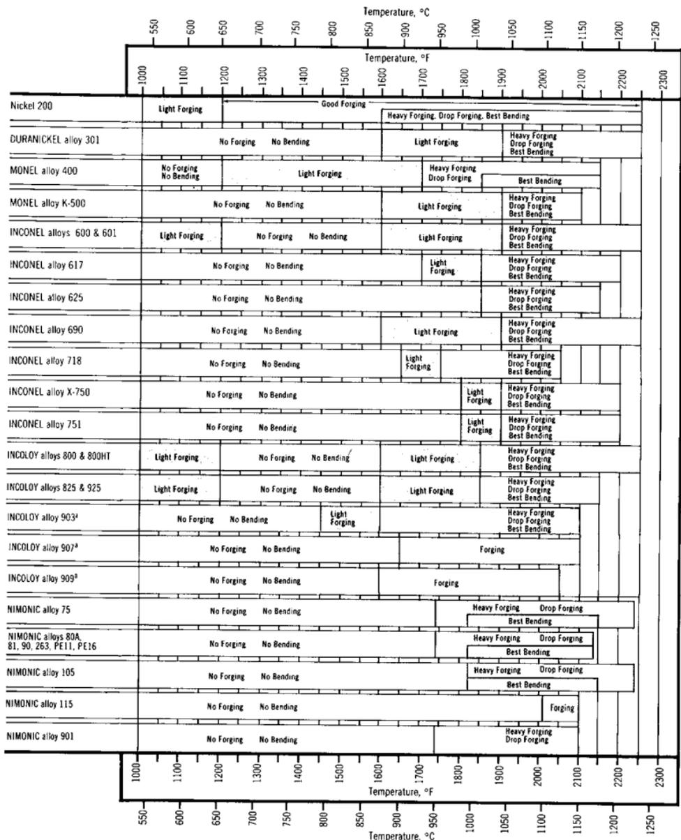
Figure 20. Temperature ranges for hot forming.
