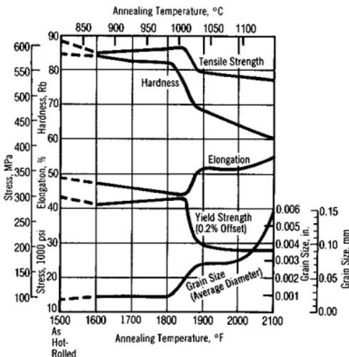
Figure 18. Effect of 15-min anneal on the grain size and room-temperature mechanical properties of an INCOLOY alloy 800 hot-rolled round 1 7/8 in. (31 mm) in diameter.
