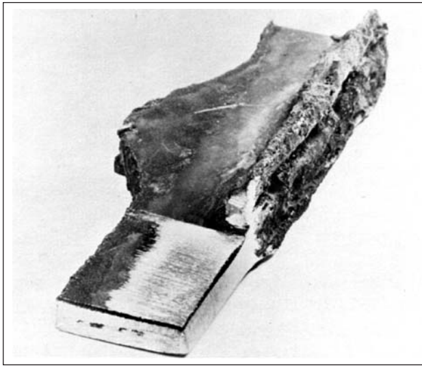
Figure 33. Iron oxide and burned material adhering to nickel alloy cut by powder-cutting process.
