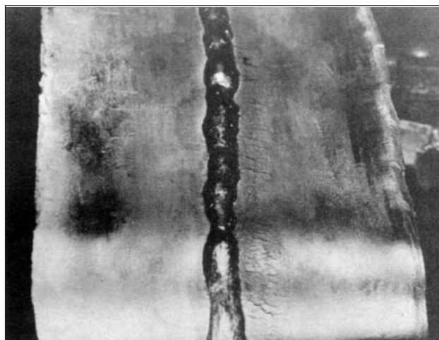
Figure 1. Sulfur embrittlement of root bend in Nickel 200 sheet. Left side of joint cleaned with solvent and clean cloth before welding; right side cleaned with solvent and dirty cloth exhibits cracking.
