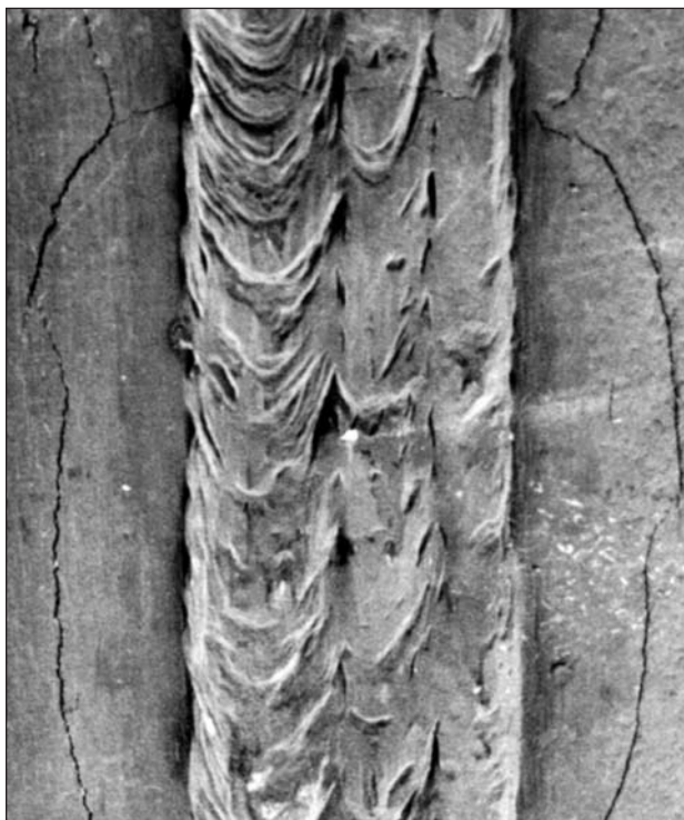
Figure 20. Failure in INCONEL alloy X-750 induced by residual welding stress at a 2-in. (51-mm) thick joint which was welded in the age-hardened condition and re-aged at 1300°F (705°C) for 20 h after welding.
