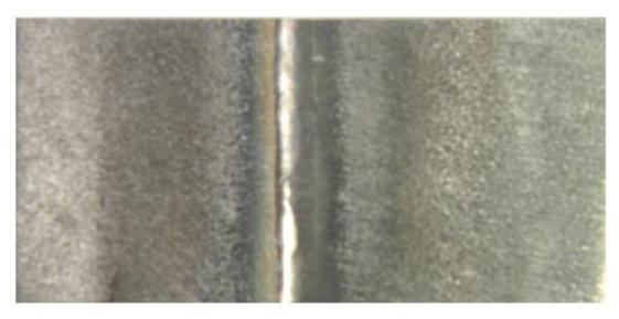
Figure 3b: Root of weld in 25-6Mo plate welded with 625 filler metal (G48A at +50°C for 24 hours) - Pitting resistance of welds in super austenitic steels.
