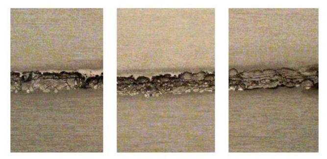
Figure 1c: INCONEL C-276 welded with INCO-WELD C-276 filler metal (pitting resistance of various base metal and weld metal combinations).
