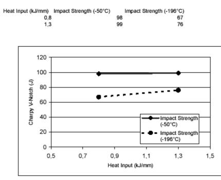
Figure 5: Variation in weld impact toughness properties for INCO-WELD 686CPT.
