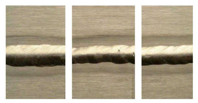
Figure 1b: INCONEL 622 welded with INCO-WELD 686CPT filler metal (pitting resistance of various base metal and weld metal combinations).
