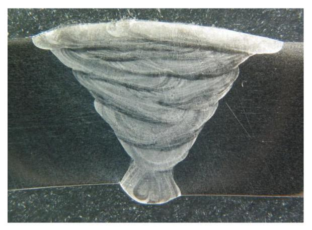
Figure 2: Macro section from a TIG weld in super austenitic stainless steel.
