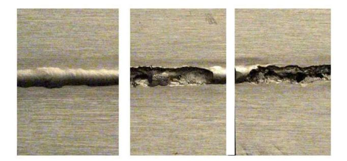
Figure 1a: INCONEL 622 welded with INCONEL 622 filler metal (pitting resistance of various base metal and weld metal combinations).
