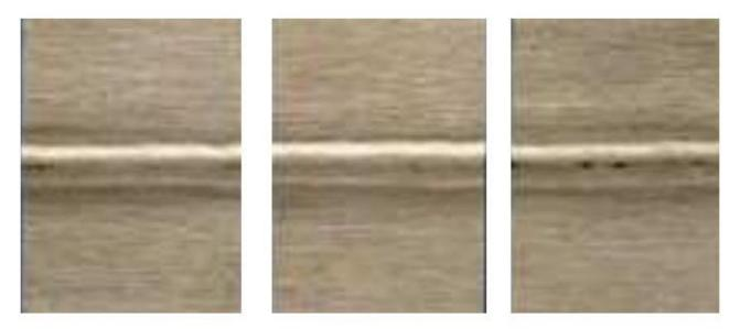
Figure 1d: INCONEL C-276 welded with INCO-WELD 686CPT filler metal (pitting resistance of various base metal and weld metal combinations).
