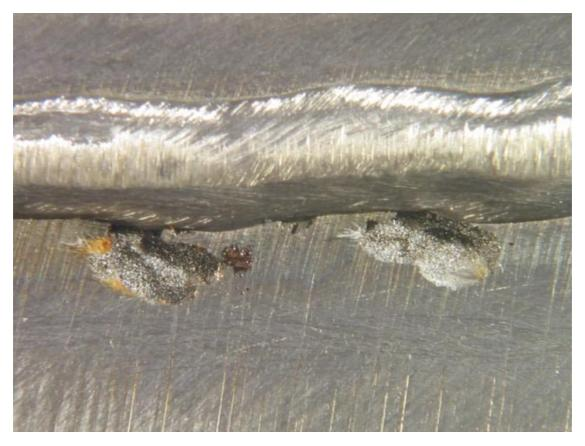
Figure 3a: Root of weld in 27-7Mo plate showing pitting in HAZ (G48C at +70°C for 24hours) - Pitting resistance of welds in super austenitic steels.
