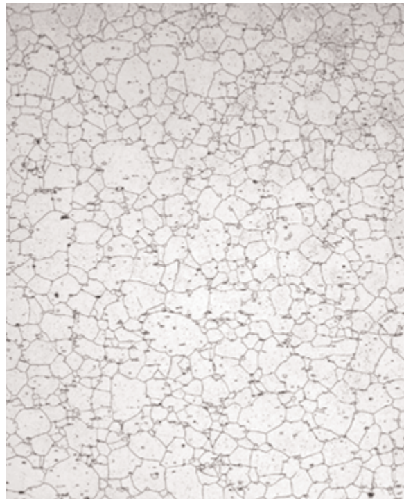
Figure 4. Photomicrograph of INCONEL alloy N06230.
