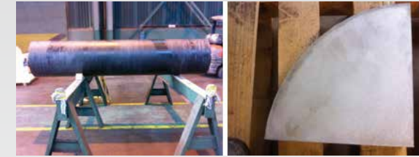
Figure 3 shows a Packer made out of alloy 945X intended for use in aggressive environment for an oil and gas well.
